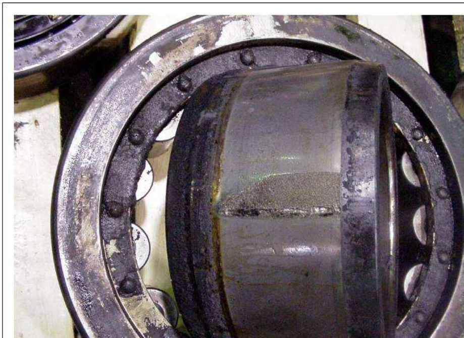
Figure 3: Damaged bearing from roller mill gearbox.
