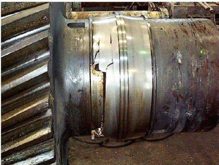
Figure 5: Defective inner race from output shaft turning at 150 RPM of pinion stand gearbox.
