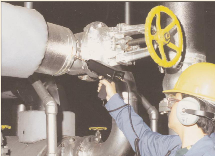
Figure 1. Ultrasound is a localized signal that makes detecting a leaking valve relatively easy. Sound levels are compared upstream vs. downstream. A louder downstream sound will indicate a leak.
