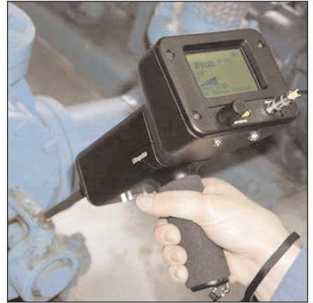
Figure 3. Some ultrasonic translators can log test results such as decibel and frequency readings. The heterodyned signal can be used to record sound samples or to connect directly to vibration analyzers for detailed spectral or time series analysis.
