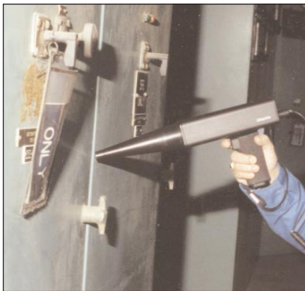
Figure 5. Arcing, tracking, corona, and partial discharge produce ionization. Inspectors can identify the type of problem based on the sound patterns. Enclosed systems can be tested by scanning door seams and air vents. A contact probe can be used on totally enclosed systems.
