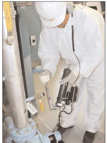
Figure 4. Overlubrication is one of the most common causes of bearing failure. To prevent this, when bearings are identified for lubrication, technicians can use ultrasonic translators to listen while the lubricant is applied and recognize when to stop lubricating.
