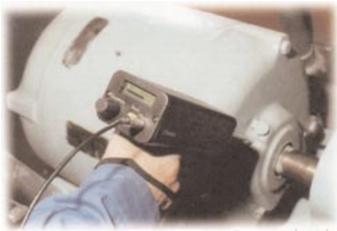
Checking grease levels using ultrasonic leak detector.
