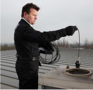
Fig. 5: Inspections using camera cable from above
