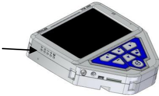
Fig. 15: openings for adjusting the monitor settings
