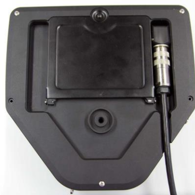
Fig. 9: Camera cable fed through guide
